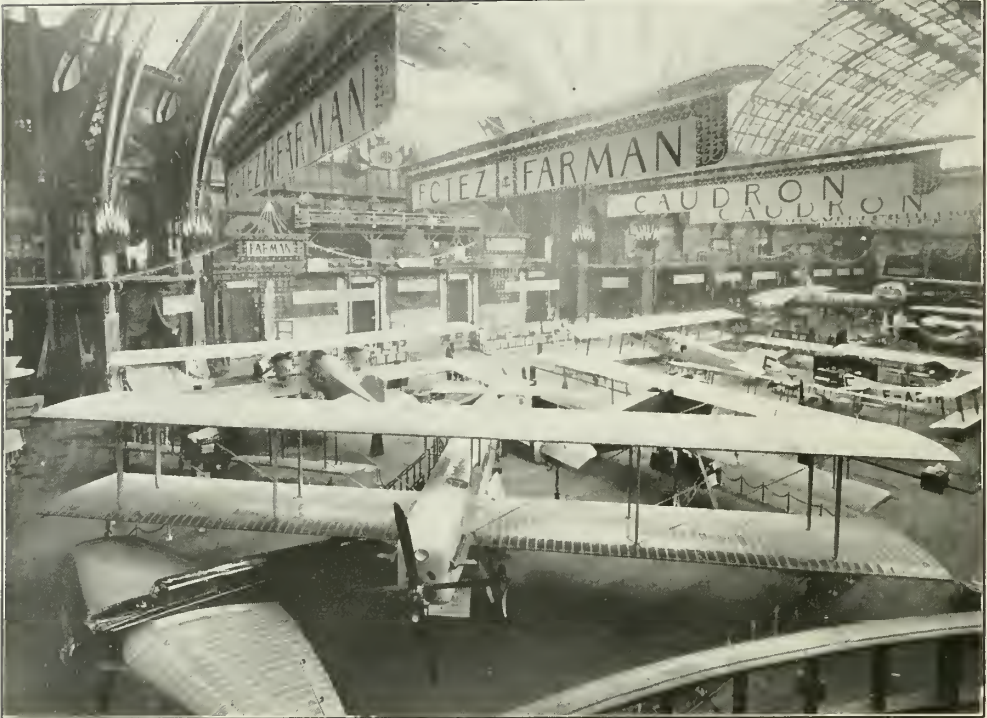
The new Farman Transport plane with one 600 h.p. motor. The single motored type is rapidly replacing the old twin-motored type in Europe
